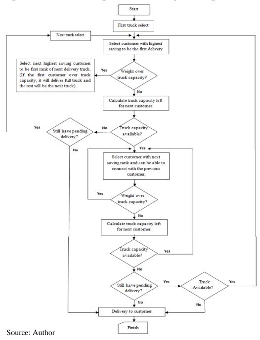
Figure 2: Process of Modeling the Vehicle Route by the Savings Method
