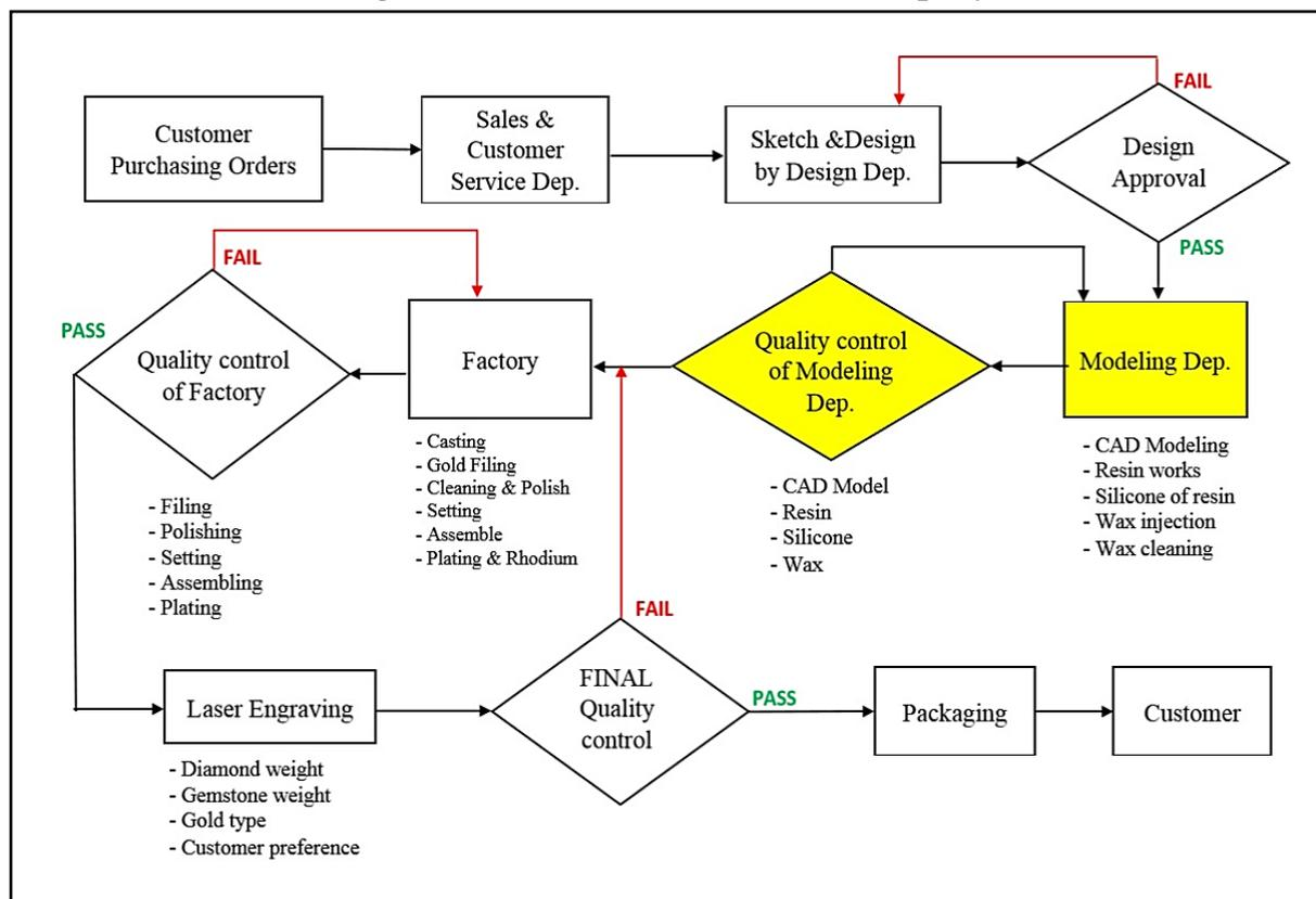
Figure 2 above shows the processes mapping of the company starting from receiving the order until it’s delivered to customers. This is only an overall process to give a holistic view of production processes. As seen in the diagram, every process needs to pass the quality control in order to continue to the next process. Processes are highlighted yellow in figure above which helps to clarify specific scope of the research.
